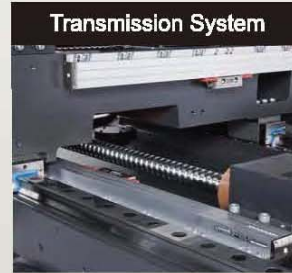
B, C Axes Worktable
