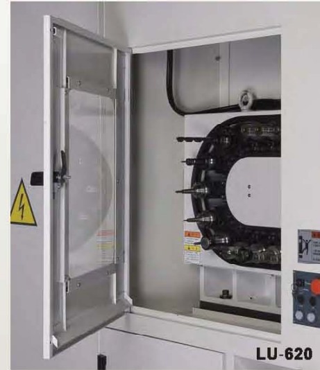
■ Magazine with maintenance door, easy for loading and unloading tools, for easy maintenance.
