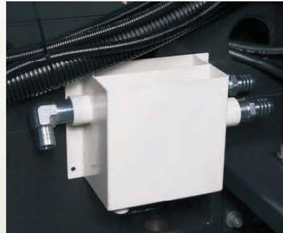
Oil-Coolant Separation Tank OP
