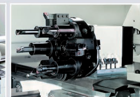
Sauter turret for static tools
