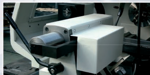
Hydraulic tailstock as an option. Quill diameter 100mm and specially extended neck. Thanks this solution there is easy access for machining close to the tailstock's centre and high rigidity of total construction.
