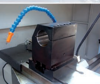
Boring bar attachment mounted on T-slots
