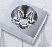
■ Process: Bottle mold ■ Workpiece: NAK-80
