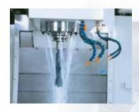
■ Eight splash nozzles on the ring surround the spindle. The splash coolant takes away heat from tool and workpiece to increase the cutting accuracy.
