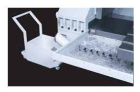
A simple but efficient removal mechanism can easily convey the chips to the rear side of the machine. The chips cart is convenient for chips disposal.
