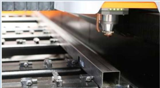
An automatic profile alignment system has been developed for precise profile cutting with a profile cutting table in machines with Fibermak pipe and profile cutting options. This feature prevents measurement drifts that may occur in profile cuts.
