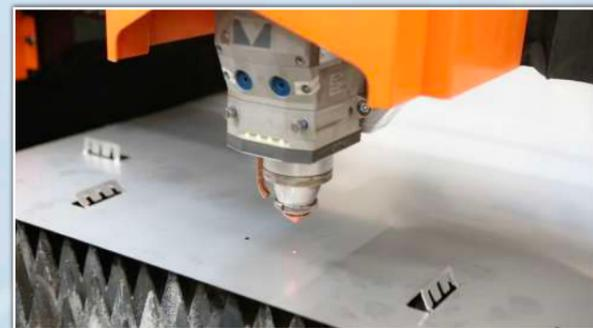
During cutting, possible collision between the laser cutting head and the displaced pieces is prevented, protecting the cutting head against damages. This feature ensures maximum safety while reducing downtime and hardware costs
