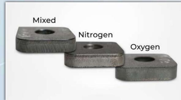
We combine the advantages of cutting processes with a mixture of nitrogen and oxygen. We provide higher speeds and excellent quality with mixed gas and as well as lower gas cost.
