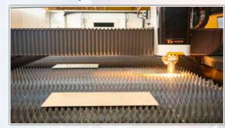
It allows the part to be cut to be sent to the cutting by selecting the sheet detected by the camera. (Auto Sheet)
