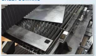
Sheet metal separation is performed on the X or Y coordinate of the selected point on the image. If there is an obstacle to cutting at the point selected by the image processing method, the cutting offset is made by detecting it on the image.
