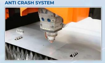
During cutting, possible collision between the laser cutting head and the displaced pieces is prevented, protecting the cutting head against damages. This feature ensures maximum safety while reducing downtime and hardware costs
