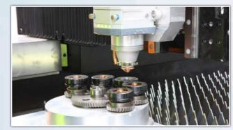
Different types of nozzles with different diameters must be used before cutting materials of different types and thickness. According to the selected sheet thickness and type, the system automatically selects and changes the defined nozzle.
