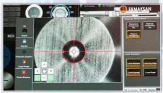
The camera-aided laser beam centering adjustment system enables the operators to adjust the laser center effortlessly when needed. Laser center adjustment camera is installed into the interior of the machine and this feature is activated by pressing a single button on the operator panel.
