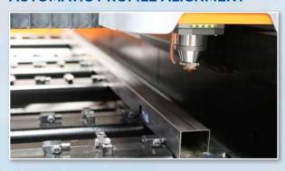
An automatic profile alignment system has been developed for precise profile cutting with a profile cutting table in machines with Fibermak pipe and profile cutting options. This feature prevents measurement drifts that may occur in profile
