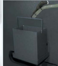
Built-in lub. oil collection system
