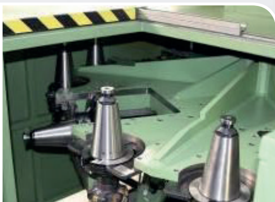
The milling head is integrated with an automated tool changer.
