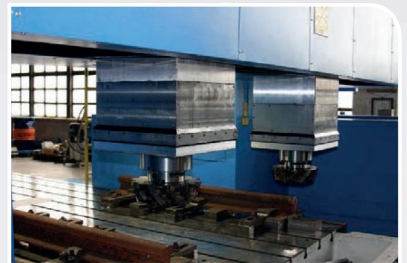
TUR RM 240 with two independent tool systems
