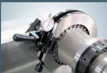
■ GN level precisely measuring clearance of spindle bearing
