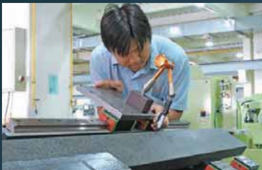
■ Flatness check for linear guide ways
