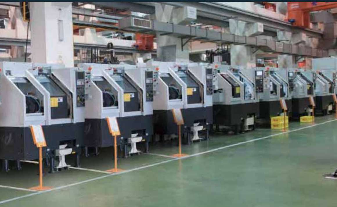
Horizontal turning center production line
