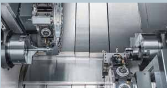
Twin spindles / Twin turrets
