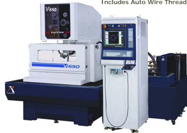
Excetek V650 Wirecut EDM Submerged Type Max workpiece size: 1000 x 700 x 405mm Max workpiece weight: 800kg Travels (X, Y, Z): 650 x 400 x 410mm Travels (U x V): 160 x 160mm Includes Auto Wire Threading
