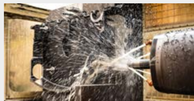
CNC Machining of cast iron saw aggregate
