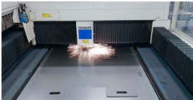
Steel plate laser cutting
