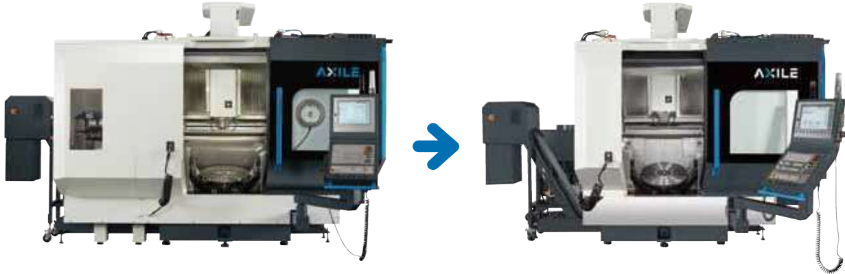
The tool magazine moves between the gantry walls
