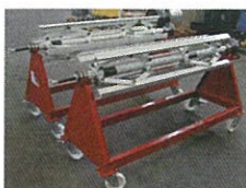
SINGLE DRUM DECOILERS AS 1250mm x 1,5 Tons
