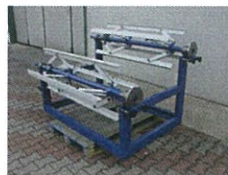
DOUBLE DRUM DECOILERS AS 2 X 1250mm X 1,5 Tons + 1,5 Tons
