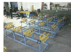
DOUBLE DRUM DECOILERS AS 2 X 1250mm X 1,5 Tons + 1,5 Tons
