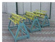
SINGLE DRUM DECOILERS AS 1250 x 5 Tons
