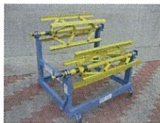
DOUBLE DRUM DECOILERS AS 2 X 1250mm X 1,5 Tons + 1,5 Tons
