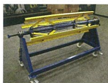
SINGLE DRUM DECOILERS AS 1250mm x 1,5 Tons
