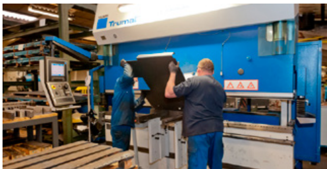
Computer assisted steel plate bending
