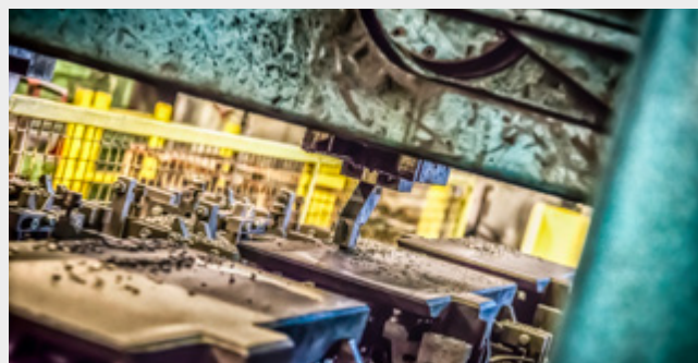
Surface planing of cast iron table
