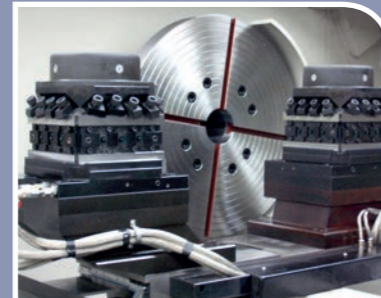
Combination of two 4-positions Sauter head-type turrets
