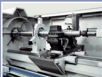
Sauter head-turret with milling unit on the rear T-slots
