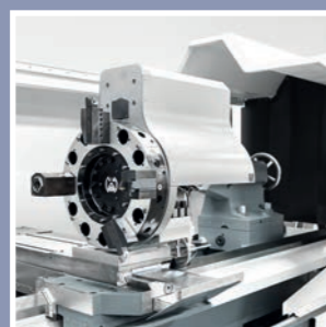
Sauter or Baruffaldi turret for driven tools with C axis
