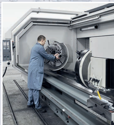
Easy access to the working area. Surprisingly small distance to spindle axis
