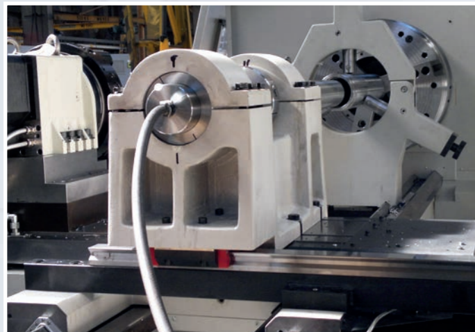
Heavy-duty boring bar attachment mounted on rear T-slots.
