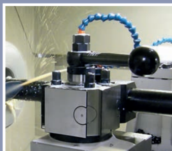
Parat toolpost with optional Capto seat
