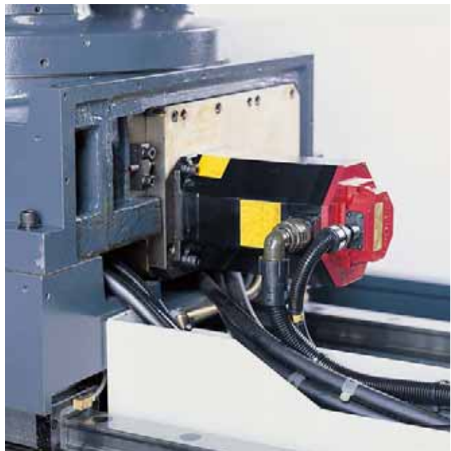
4 th axis rotary cables centralized
